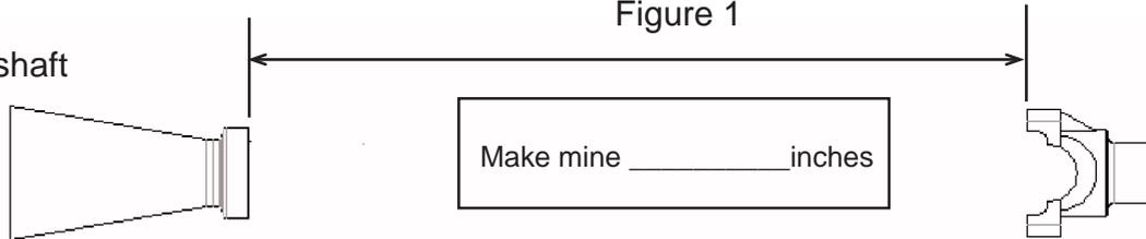
*Take all measurements with the rear housing supported at ride height!*
