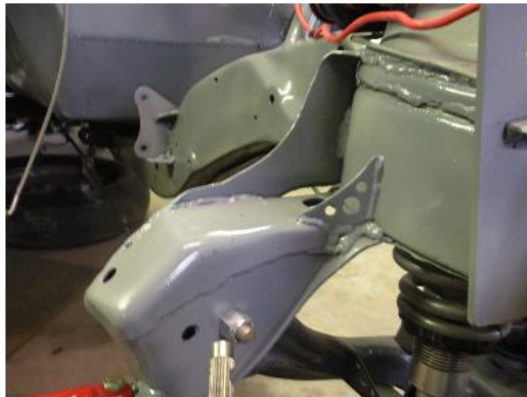
Photo B. A-arm mounting box with crossmember removed
