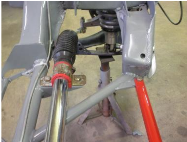
Photo D. Diagonal tubes, bolt in crossmember & tabs
