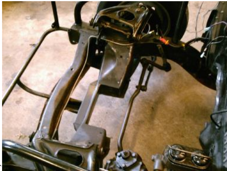
Photo A. OEM steering box & linkage, front crossmember & modified rear crossmember
