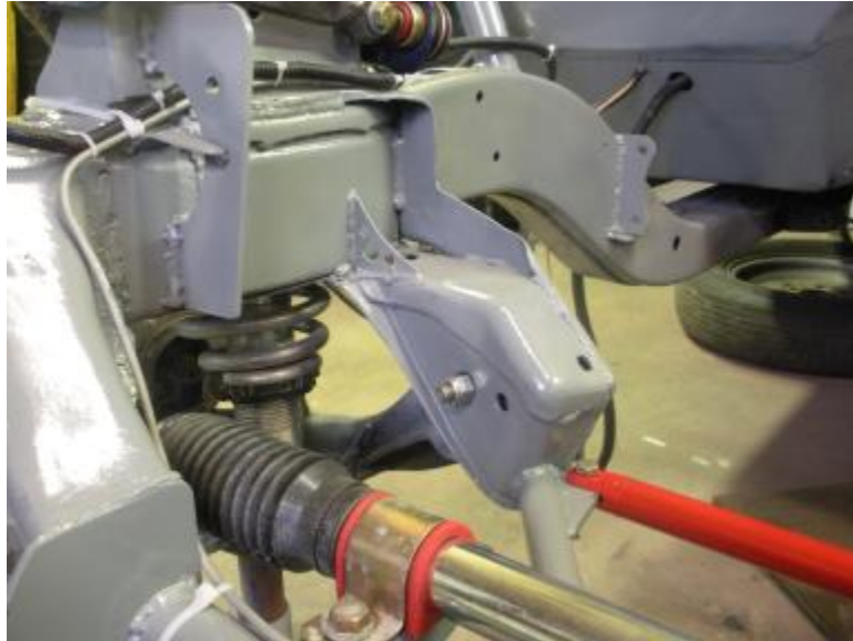
Photo C. Passenger side a-arm mounting box
