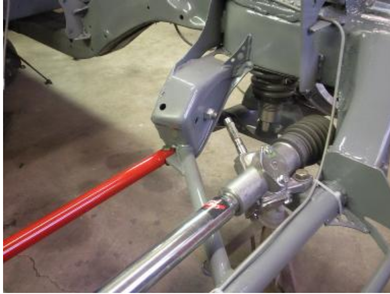
Photo E. Note location of 1/8" plate gussets
