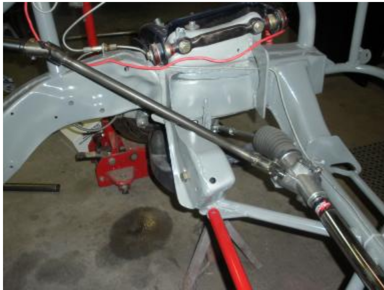
Photo F. Locate R&P so that steering shaft does not rub A-Arm mount
