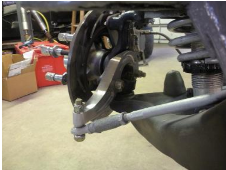
Photo H. Tie rod ends & steering arms
