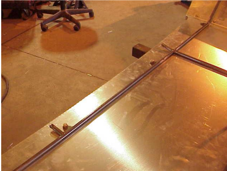
Figure 3 Clevis attaches to trunk brackets
